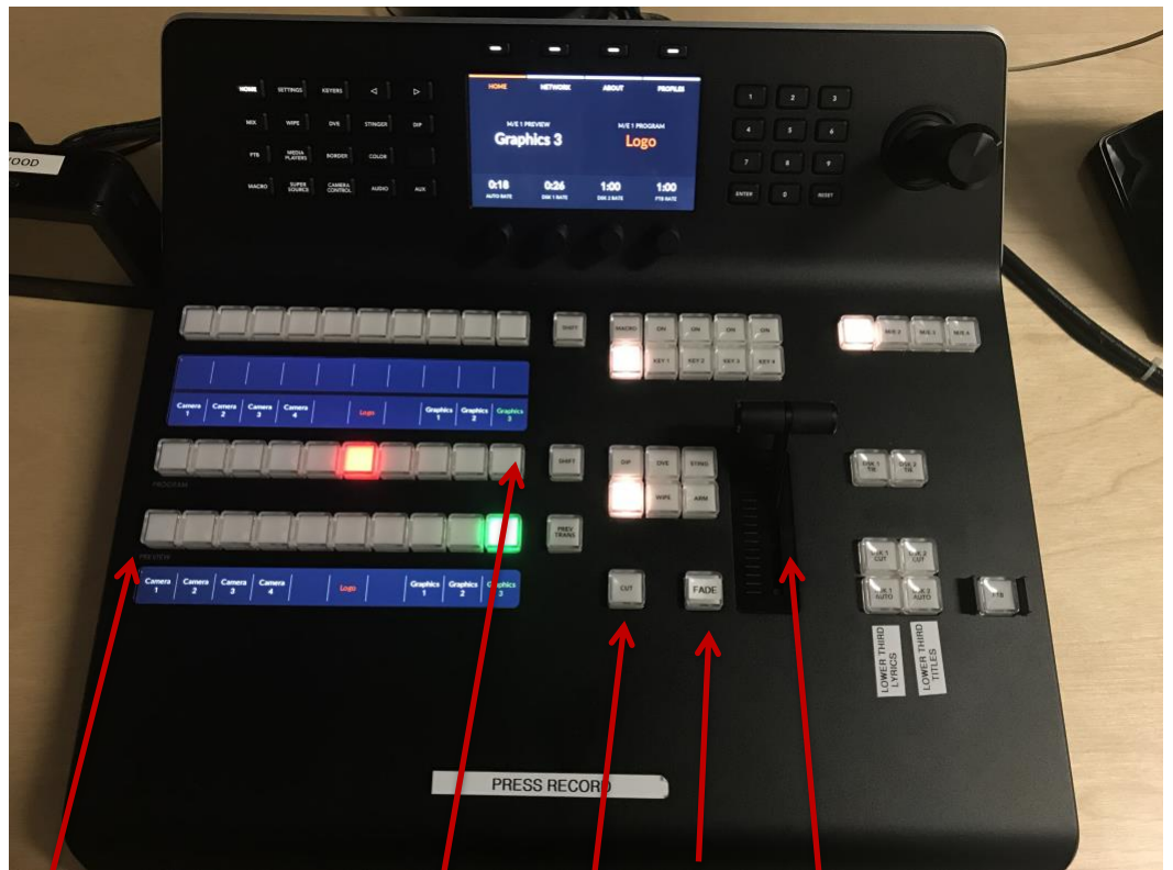
PREVIEW row GREEN. View on the PREVIEW screen. PROGRAM row (6) RED. View on the live PROGRAM screen (7) CUT (8) FADE DISSOLVE
